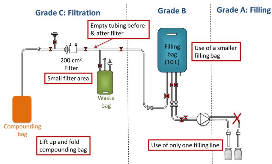
Figure 1. Strategies for minimizing losses with the existing fill set-up.
